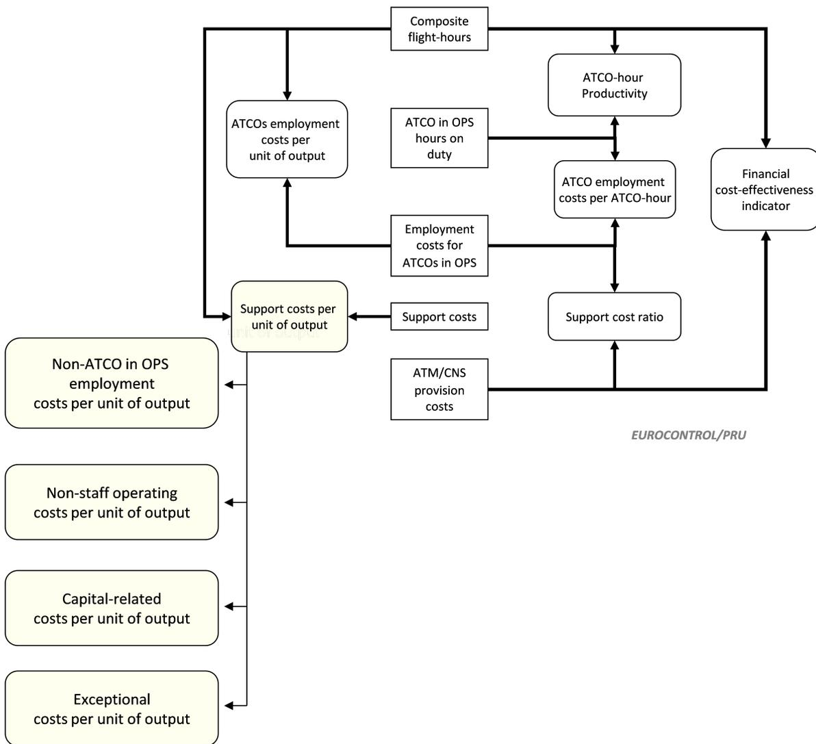
Figure 3.1: Performance framework for gate-to-gate cost-effectiveness analysis
